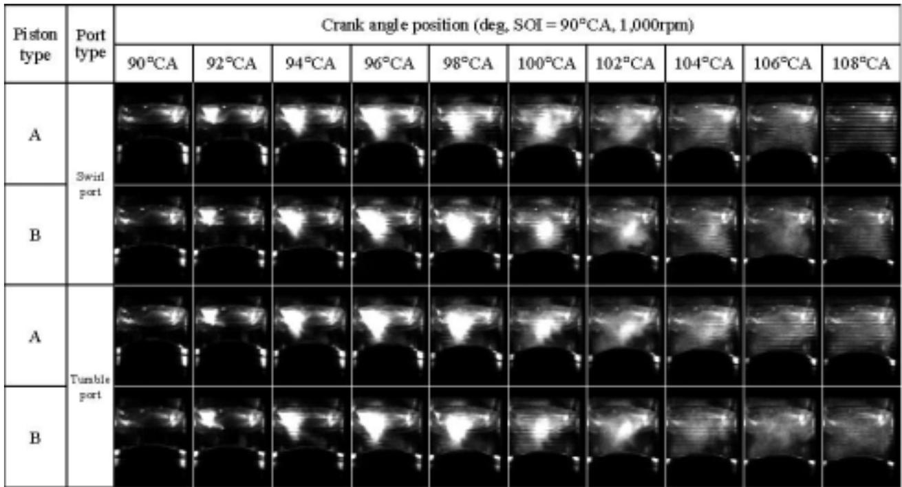
Figure 9 In-cylinder spray flow visualization at ATDC 90° fuel injection
