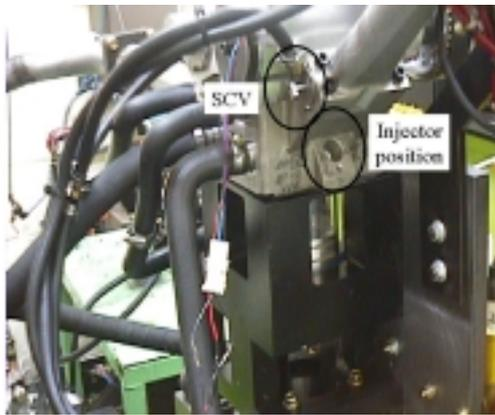
Figure 2. Photography of SCV and Injector position
