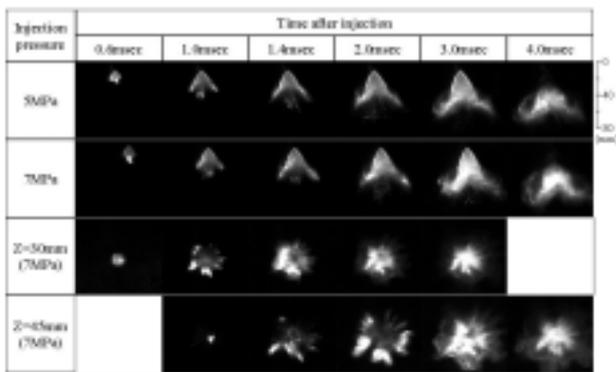
Figure 6. Spray developments and overall structure of the high-pressure swirl-type gasoline injector
