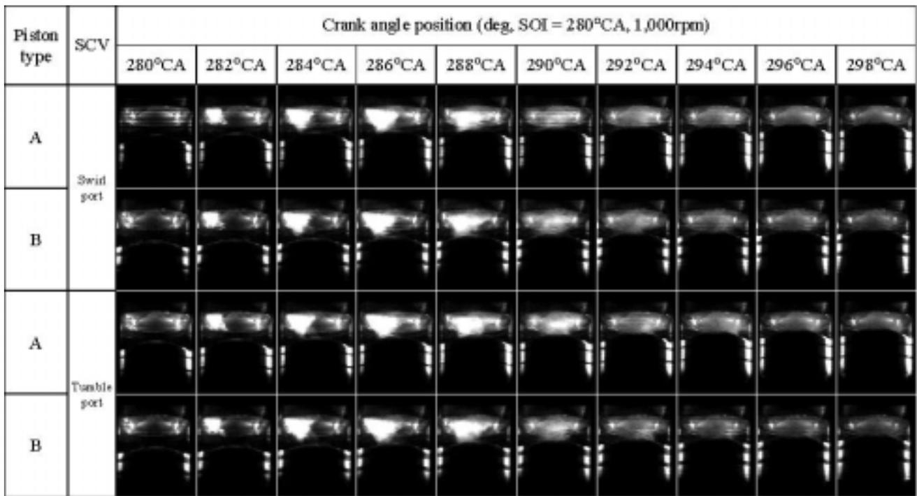
Figure 11 In-cylinder spray flow visualization at ATDC 280° fuel injection
