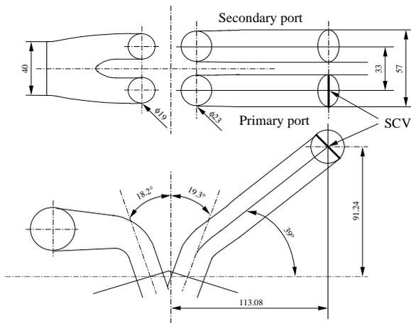
Figure 1. Intake port geometry of GDI engine
