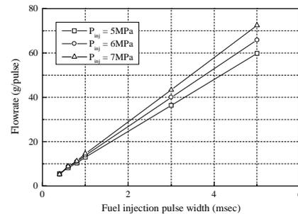
Figure 5. Effect of injection pressure on injection flowrate with different fuel injection pulse width
