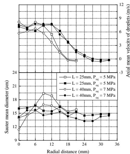
Figure 8. Radial distribution of SMD and axial mean velocity at different axial distance
