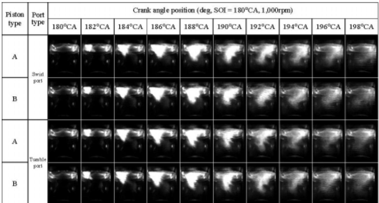
Figure 10 In-cylinder spray flow visualization at ATDC 180° fuel injection
