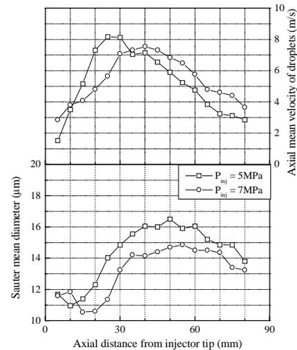
Figure 7. Axial distribution of SMD and axial mean velocity at the center of injection axis
